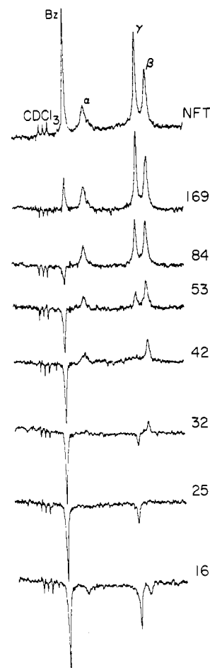
FIGURE 6: Saturated carbon region in the proton-decoupled natural-abundance 13 C PRFT nmr spectra of helical (BzlGlu) n of mol wt 17,000 at 40°, recorded at 14.2 kG using 512 accumulations with a recycle time of 1.1 sec. Solvent and concentration are the same as in Figure 4A. Number next to each spectrum is the interval between each 180° radiofrequency pulse and the following 90° pulse, in msec. The normal Fourier transform spectrum (NFT) shown on top is one obtained in the absence of 180° pulses.
